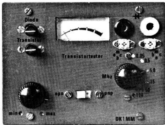
Fig. 1: The prototype bi-polar transistor tester as built by Martin Michaelis DK1MM.
